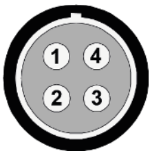
Figure 4: Pin assignment trigger (socket view, device)
