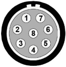
Figure 5: Pin assignment trailing cable box (socket view, device)
