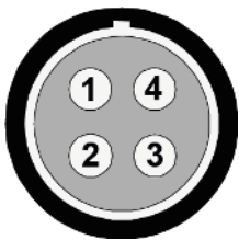
Figure 2: Pin assignment power (socket view, device)
