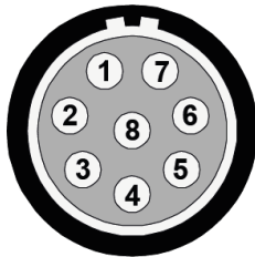
Figure 5: Pin assignment trailing cable box (socket view, device) Use this plug: LEMO FGB.1B.308...
