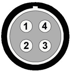
Figure 1: Pin assignment power input (socket view, device)
