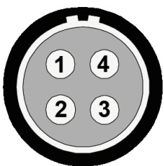
Figure 2: Pin assignment power output (socket view, device)
