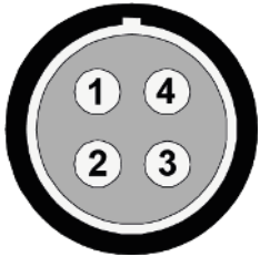
Figure 5: Pin assignment power (socket view, cable)
