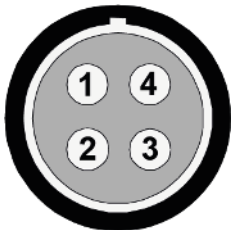
Figure 1: Pin assignment release connector for fire or safe (socket view, device)
