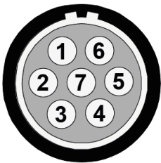
Figure 1: (MESSRING product code 4ADA621) Pin assignment, connector 1 (socket view, device) Use this plug: LEMO FGA.1B.307...
