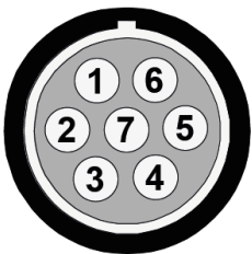
Figure 2: (MESSRING product code 4ADA621) Pin assignment, connector 2-8 (socket view, device) Use this plug: LEMO FGG.1B.307...
