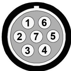
Figure 2: (MESSRING product code 4ADA621) Pin assignment, connector 2-8 (socket view, device)
