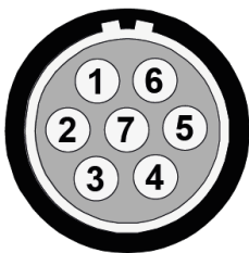
Figure 1: (MESSRING product code 4ADA621) Pin assignment, connector 1 (socket view, device)
