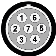
Figure 2: (MESSRING product code 4ADA612) NA3x pin assignment (socket view, device)
