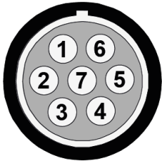
Figure 3: (MESSRING product code 4ADA618) CP pin assignment (socket view, device) Use this plug: LEMO FGG.1B.307...
