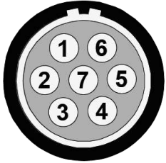
Figure 1: Pin assignment USB connection (socket view, device) Use this plug: LEMO FGB.1B.307...
