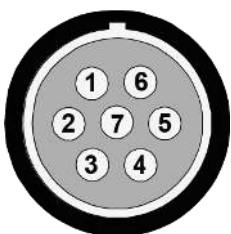
Figure 2: (MESSRING product code 4BBD212) NA3X pin assignment (socket view, device) Use this plug: LEMO FGG.1B.307...
