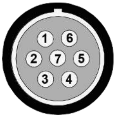
Figure 1: (MESSRING product code 4BBD211) Standard pin assignment (socket view, device) Use this plug: LEMO FGG.1B.307...
