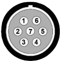
Figure 2: (MESSRING product code 4BBD212) NA3X pin assignment (socket view, device) Use this plug: LEMO FGG.1B.307...
