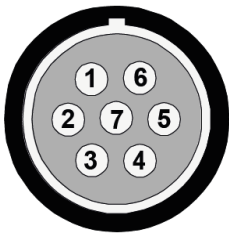
Figure 1: (MESSRING product code 4BBD211) Standard pin assignment (socket view, device) Use this plug: LEMO FGG.1B.307...
