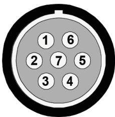
Figure 3: (MESSRING product code 4BBD214) CP pin assignment (socket view, device) Use this plug: LEMO FGG.1B.307...
