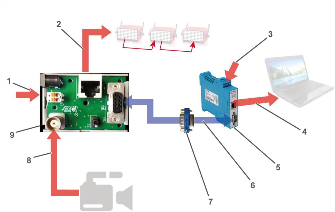
Figure 4: M=LIGHT installation set for stationary installation (schema)
