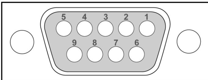
Figure 26: DB9 female connector for CAN@net II Interface Adapter
