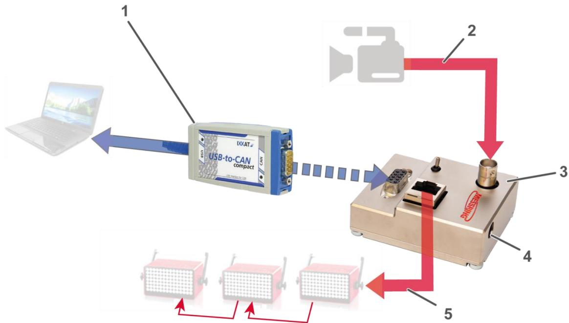
Figure 2: Connection M=LIGHT, camera and PC (schema)
