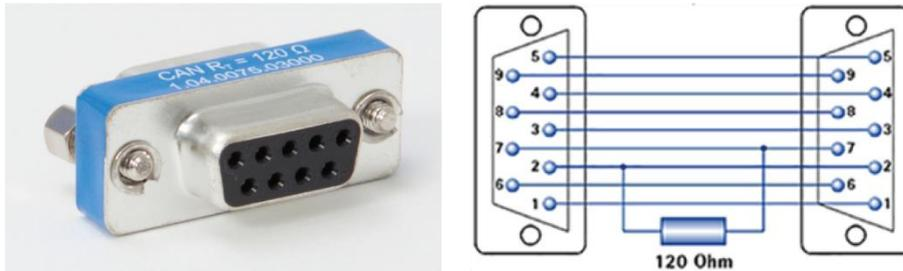
Figure 32: Bus terminator and connections of the bus terminator
