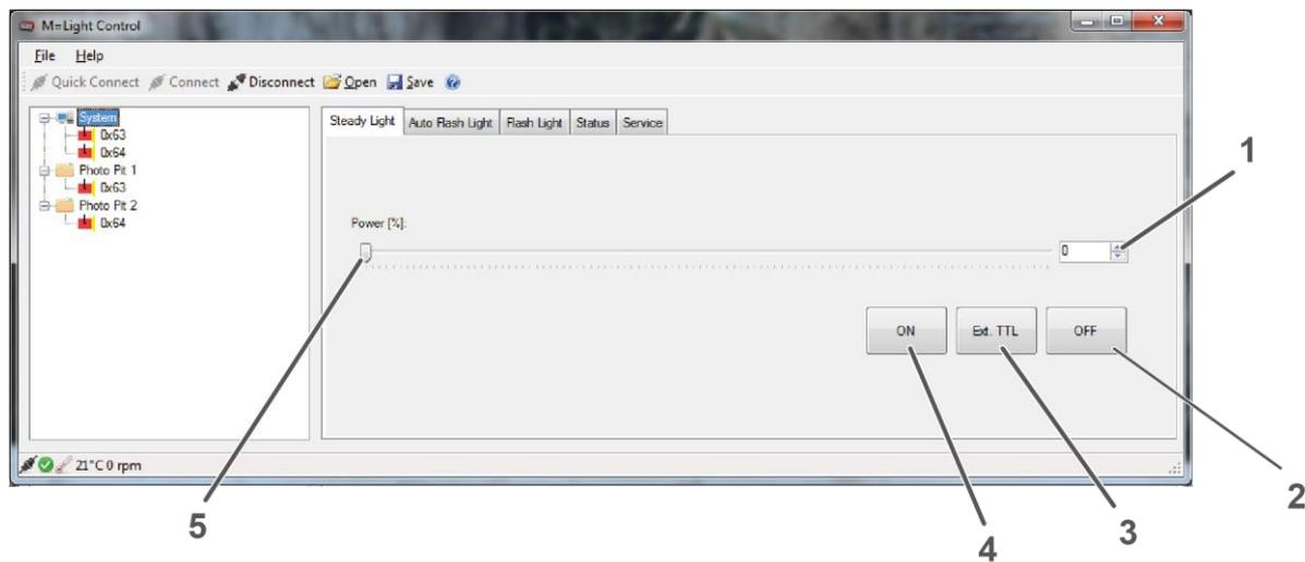
Figure 44: Steady light tab
