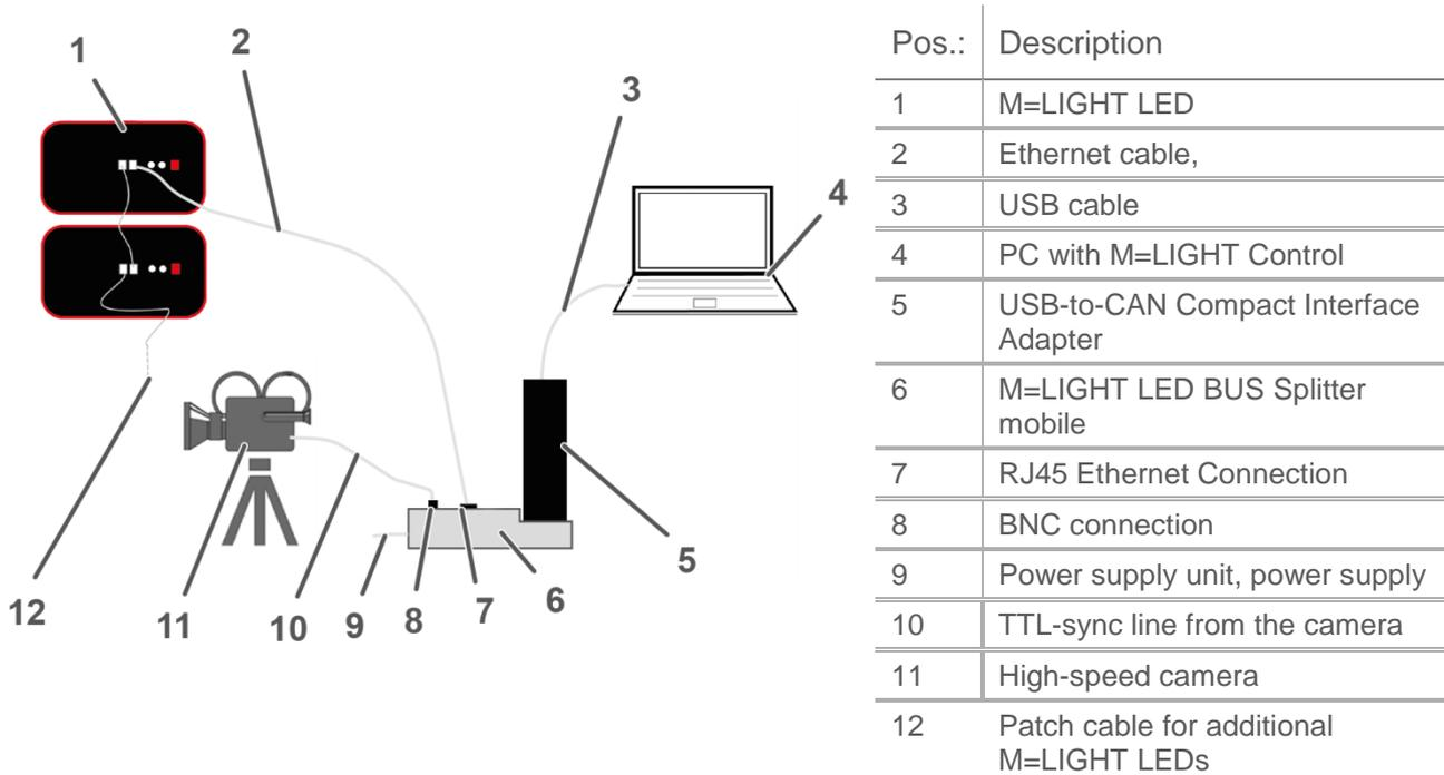
Figure 62: Connection M=LIGHT LED, (schematic diagram)
