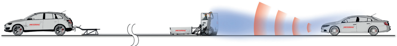
Figure 2: Test situation: SprayMaker mounted on common vehicle target (Euro NCAP Vehicle)
