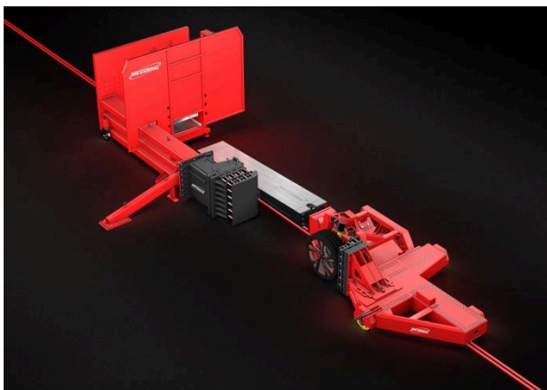
Illustration of the M=SLED Small Overlap right before the impact on the force measurement wall
