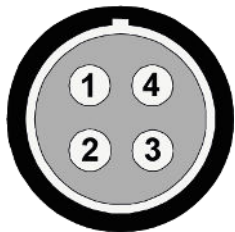
Figure 5: Pin assignment power (socket view, cable)
