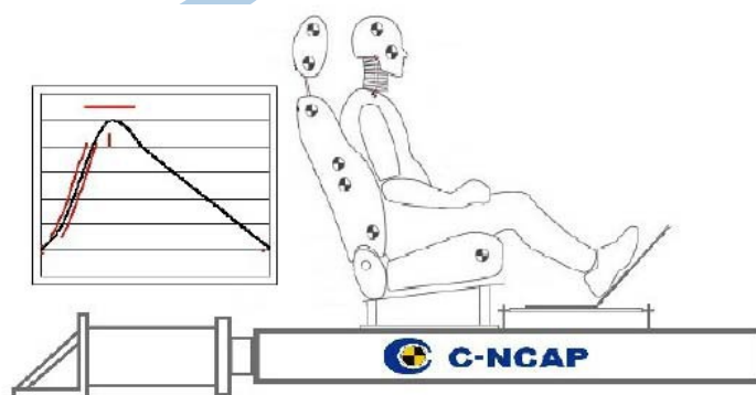
Figure 4 Neck protection test in low-speed rear impact (whiplash test)
