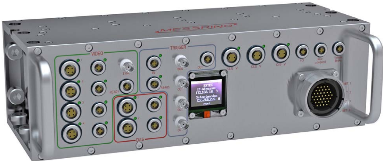
Trailing cable connector box at vehicle/sled 3AK-C31-1
